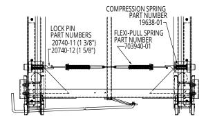
Lockpins with Flexipull - CURRENT PRODUCTION Used on sliders with production date after 2-1-03
