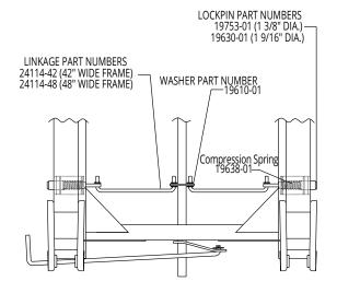
Lockpins with Slot Attachment Used on sliders with production dates prior to 2-1-2000 K704550 - Flexi-Pull Conversion Kit
