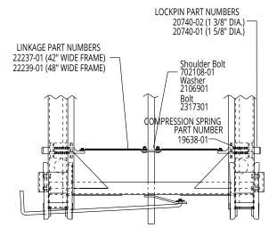
Lockpins with "T" Post Attachment Used on sliders with production dates from 2-1-2000 - 2-1-2003
