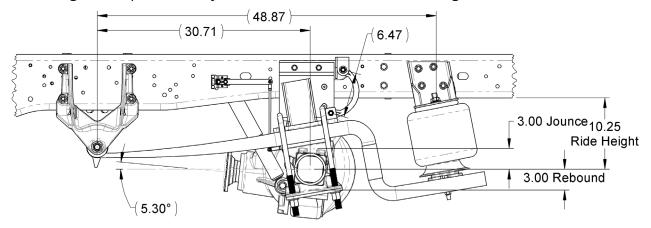
Figure 1: Suspension range of motion
