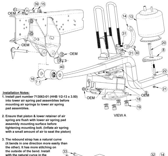
The rebound strap has a natural curve (it bends in one direction more easily than the other). It has more stitching on the outside of the bend. Install with the natural curve in the position shown
