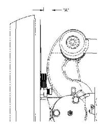
Figure 12 - Steering Stop Bolt
