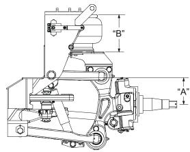
Figure 11 – Measurement at Ride Height
