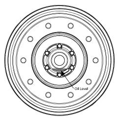
Figure 18 - Wheel Bearing Oil Level
