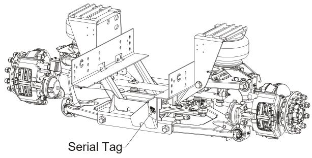
Figure 1 - Suspension Identification Location
