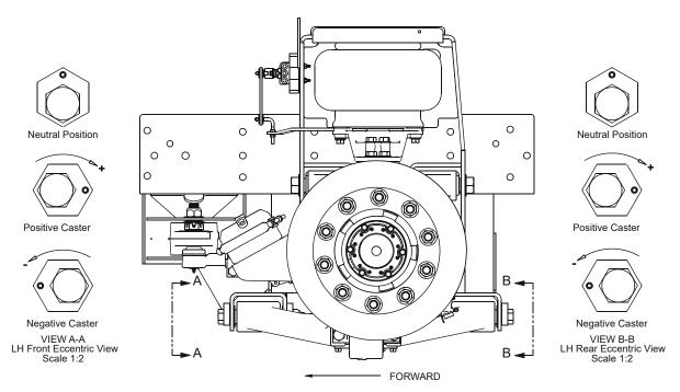
Figure 17 – Eccentric Caster Adjustment
