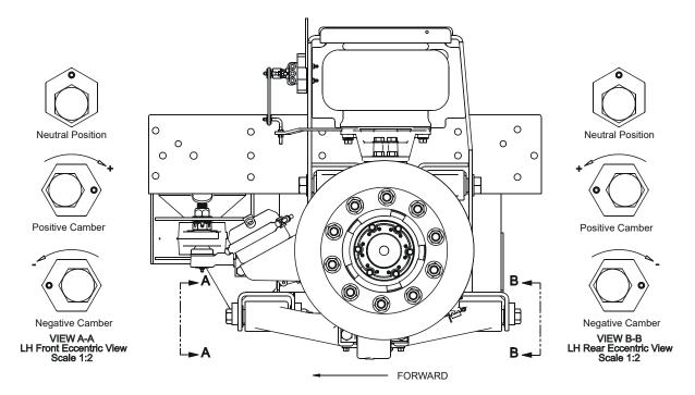
Figure 14 – Eccentric Camber Adjustment
