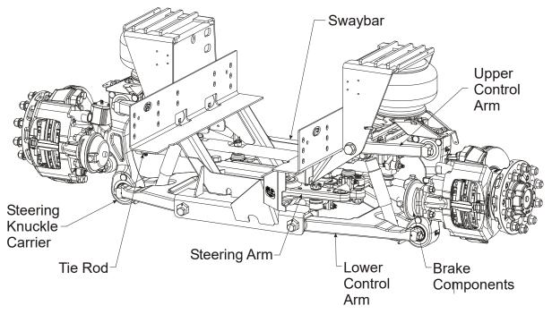
Figure 3 – Improper Tow Equipment Attachment Locations
