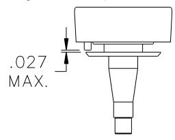
Figure 7 - ABS Sensor and Tone Ring Gap
