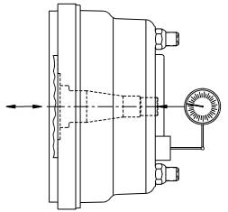
Figure 10 - Wheel End Play Measurement
