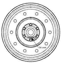
Figure 5 - Wheel Bearing Oil Level
