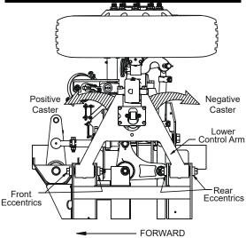
Figure 16 – Lower control arm movement
