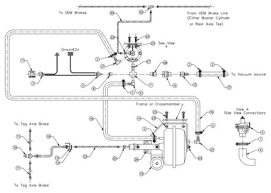
Note: The large 90° hose, item 6, attached to the bottom of the synchronizing valve, item 4, should be directed rearward and away from the rear tires to prevent road spray entering the synchronizing valve.
