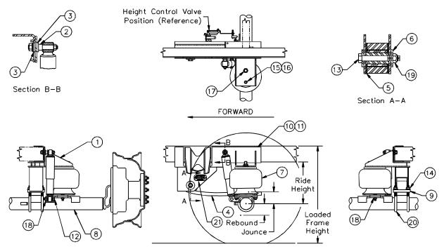
Note: The ride height is for the completed vehicle with body and components. See table below for correct vehicle dimensions.
