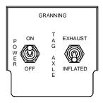
Figure 2: Control Panel Assembly, 4555, with Power and Kneeler Option
