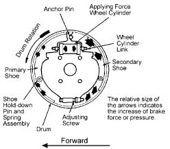
Figure 9: Brake Backing Plate Detail
