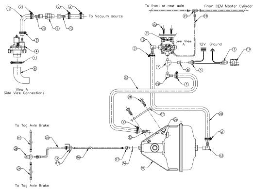
Note: The large 90° hose, item 6, attached to the bottom of the synchronizing valve, item 4, should be directed rearward and away from the rear tires to prevent road spray entering the synchronizing valve.
