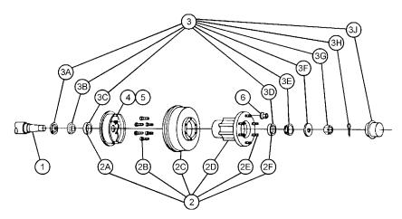
Figure 8: Hub and Drum Assembly
